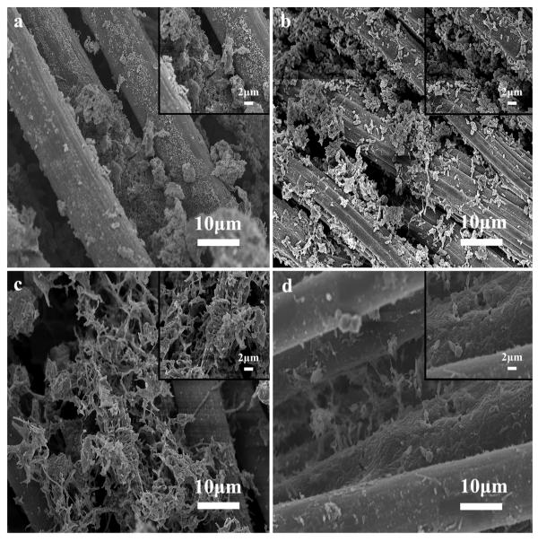
Fig. 4. SEM images of the anode biofilms treated with 0 g/L (a), 1 g/L (b), 2 g/L (c) and 4 g/L (d) lysozyme and run in MFC for 65 h.
