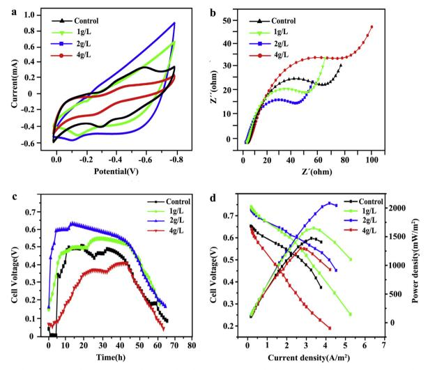
Fig. 5. Cyclic voltammograms (a), electrochemical impedance plots (b), voltage-time curves (c) and polarization curves (d) of the MFCs with the anodes treated with 0 g/L (control), 1 g/L, 2 g/L and 4 g/L lysozyme.
