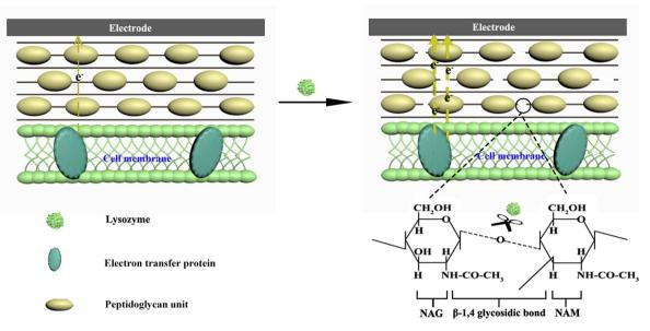
Fig. 1. Schematic preparation process of lysozyme partially hydrolyzes the peptidoglycan layer of Gram-positive bacteria in biofilms, enhancing the efficiency of electron transfer from bacteria to electrodes.
